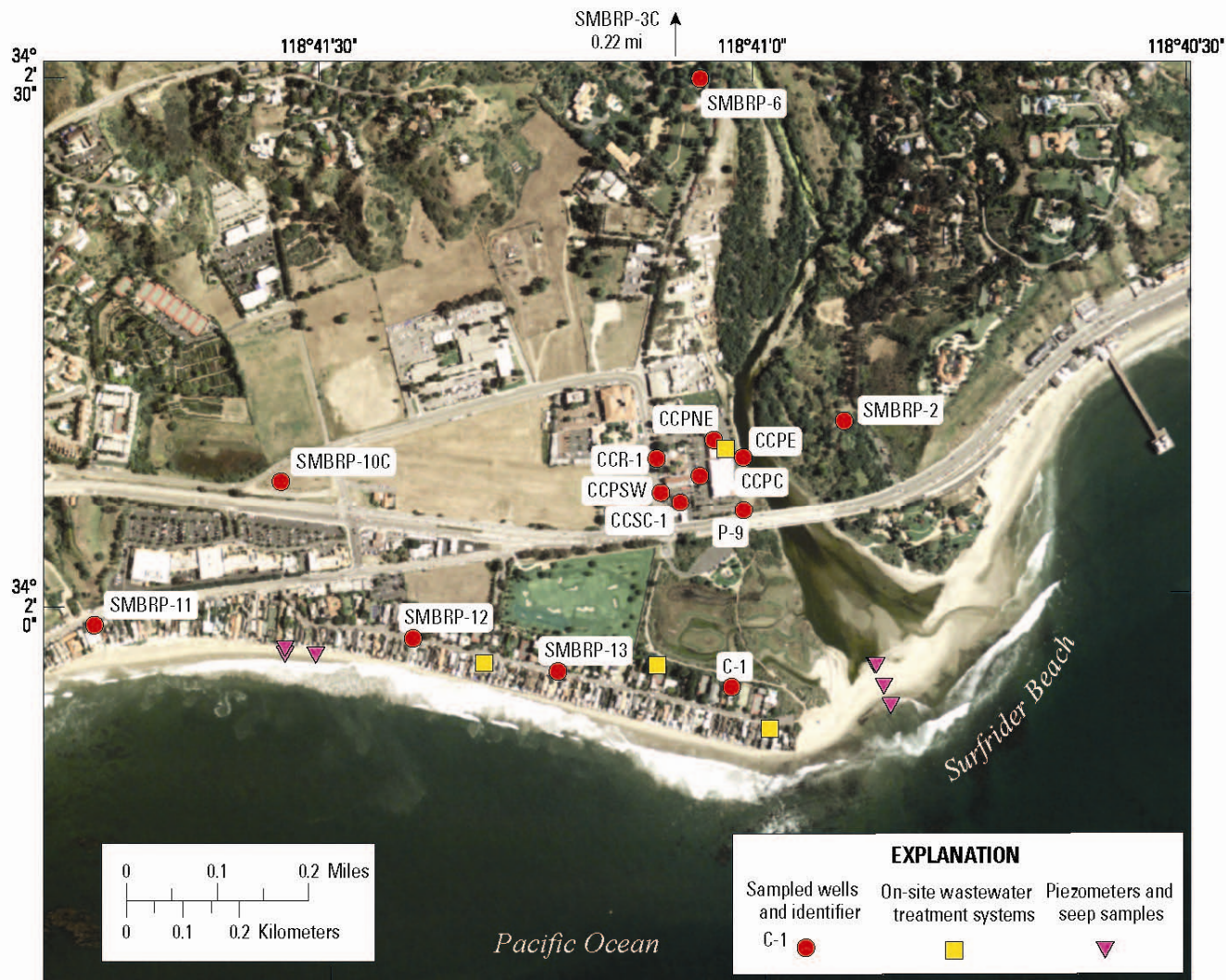
Figure 3 Location of sampled wells, piezometers, seepage samplers and onsite wastewater treatment systems (OWTS), Malibu, California, July 2009 to April 2010.
