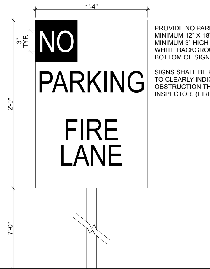
FIRE LANE PARKING SIGNAGE
